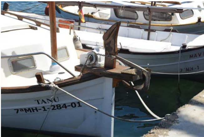
Typical Balearic Island Fishing Boat Bow Configuration
